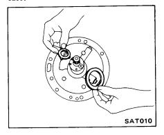
11. Back off band servo piston stem to release band.
