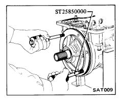
10. Remove high-reverse clutch (Front) thrust washer and bearing race.
