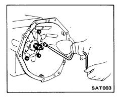
3. Unscrew and remove downshift solenoid and O-ring.
