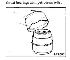
(2) Install assembly into transmission case. Check that parts are properly seated before proceeding with measurements.
