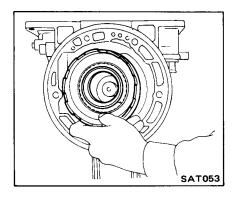
12. Install rear internal gear.
