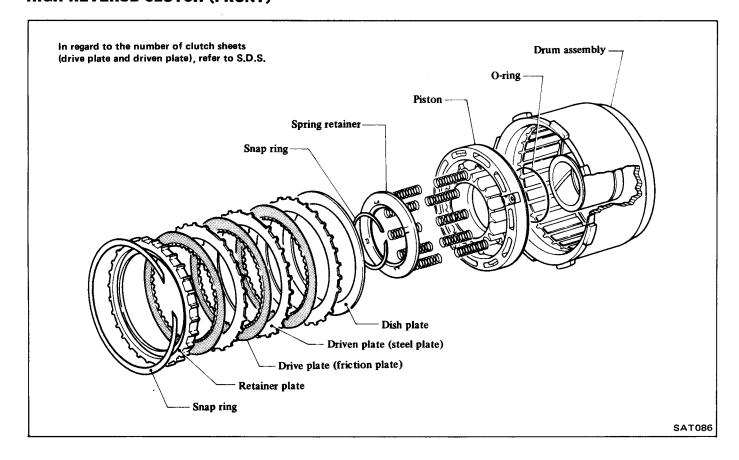
1. Using a screwdriver, remove large clutch retaining plate snap ring.
