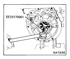
19. Pry off one end of snap ring with a screwdriver. Remove snap ring from low and reverse brake assembly while applying plier force in direction of arrow.
