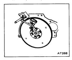
2. Installation of torque converter
