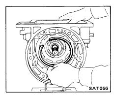
10. Install one-way sprag into one-way clutch outer race (attached to connecting drum).
