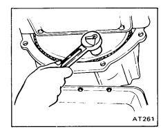
Before removing torque converter, inscribe chalk marks on two parts so that they may be replaced in their original positions at assembly.
