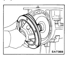
22. Adjust band. Make sure that brake band strut is correctly installed. Torque piston stem to specified value. Back off two full turns and secure with lock nut.
