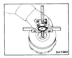
(5) Measure from top of oil pump shaft to gasket installed (dimension C).
