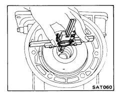
(4) Assemble high-reverse clutch (Front) and forward clutch (Rear) drum assemblies together and lay them flat on bench. Be sure rear hub thrust bearing is properly seated. Meas-
