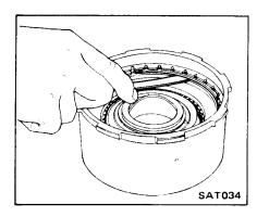
14. Testing high-reverse clutch (Front)
