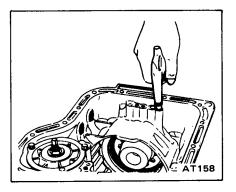
8. Install governor thrust washer and needle bearing.
