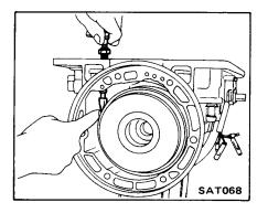
21. Mount oil pump gasket on oil pump with petroleum jelly. Align pump to transmission case and install.
