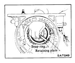
7. Using an air gun with a tapered rubber 'tip, check low and reverse brake operation.
