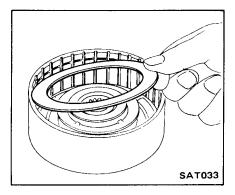
12. Now install driven plate (steel plate), then a drive plate (friction plate) and repeat in this order until correct number of plates has been installed (check Service Data and Specifications for proper quantity of plates). Now install retainer plate and snap ring.
