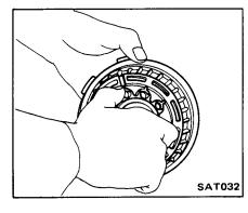
3. Compress clutch springs and remove snap ring from spring retainer.
