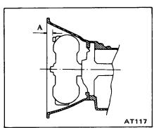
4. Bolt converter to drive plate.
