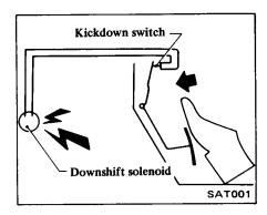
Do not allow the switch to make contact too soon. This would cause
