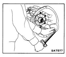
30. Before installing vacuum diaphragm valve, measure depth of hole in which it is inserted. This measurement determines correct rod length to ensure proper performance.
