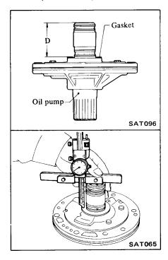
(7) Difference between dimension [A-0.1 mm (0.004 in)-B] and (C-D) is front end play and must be within specified value.
