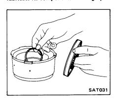
Remove clutch plate assembly.
