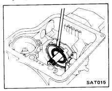
17. Remove output shaft snap ring.
