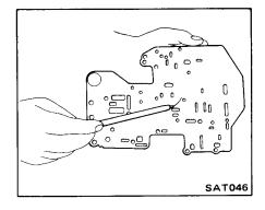
10. Check oil passages in upper and lower valve bodies for varnish deposits, scratches or other damage that would impair valve movement. Check threaded holes and related bolts and screws for stripped threads; replace as needed. 11. Test valve springs for weakened load condition. Refer to Valve Body Spring Chart for spring specifications.
