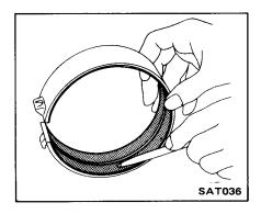
Check band servo components for wear and scoring. Replace piston O-rings and all other components as necessary.
