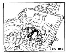
18. Remove rear connecting drum with internal (annulus) gear.
