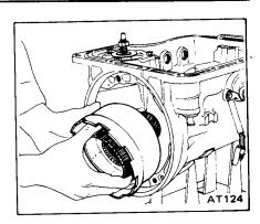
15. Back out, about half-way, band servo attaching bolts. Using an air gun, carefully apply pressure to loosen band servo. Remove band servo retaining bolts and pull band servo.
