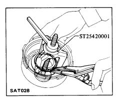
11. Install dish plate with dish facing outward.
