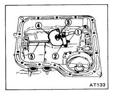
28. Remove inhibitor switch and manual shaft by loosening two securing bolts.
