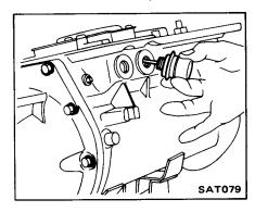
34. Install inhibitor switch. Check for proper operation in each range using a circuit tester. Refer to Minor Adjustment.
