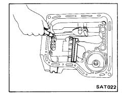
24. Remove governor thrust washer and needle bearing.
