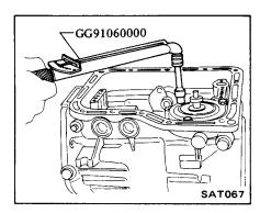
20. Finger tighten brake band servo piston stem enough to prevent brake band and strut from falling out. Do not adjust brake band at this time.
