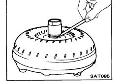
38. Lubricate oil pump lip seal and converter neck before installing converter.
