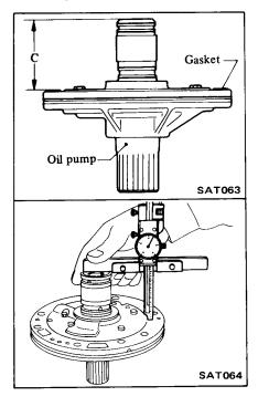
(6) Install thrust washer. Measure from top of oil pump shaft to thrust washer (dimension D).
