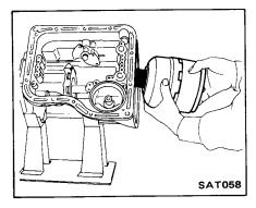
(3) Using a dial gauge or caliper with a seven inch base, measure from rear hub thrust bearing race to case (dimension A).
