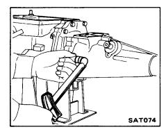
27. Install control valve body. Be sure manual valve is in alignment with selector pin.
