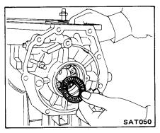
9. Slide governor distributor assembly on output shaft from front of shaft. Install shaft and governor distributor into case, using care not to damage distributor rings.
