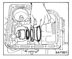
20. Tilt extension housing upward and remove low and reverse brake clutch assembly.
