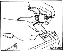
35. Before installing oil pan, check alignment and operation of control lever and parking pawl engagement. Blow mechanism with air to clean. Make final check to be sure all bolts are installed in valve body.
