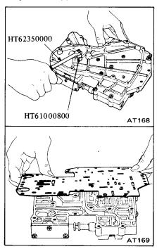
3. During valve body separation, do not scatter or lose orifice check valve, servo orifice check valve, and throttle
