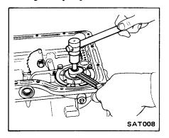
9. Remove input shaft from pump.
