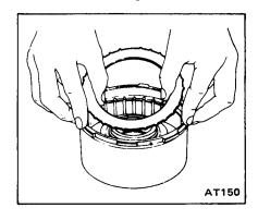
5. For easy removal of piston from drum, mount clutch on pump. Use an air gun with a tapered rubber tip to carefully apply air pressure to loosen piston from drum.
