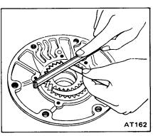
7. Measure clearance between seal ring and ring groove.
