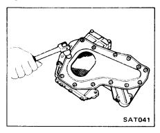
2. Disassemble valve body and its remaining attaching bolts and nuts to carefully separate lower body, separator plate and upper body.
