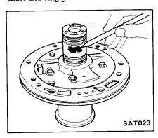
2. Remove pump cover from pump housing.
