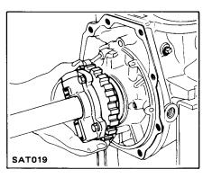
26. Using an air gun with a tapered rubber tip, carefully apply air pressure to remove low and reverse brake piston.
