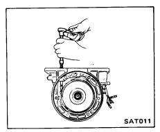
12. Remove brake band strut. Brake band, high-reverse clutch (Front) and forward clutch (Rear) assemblies may be removed together.
