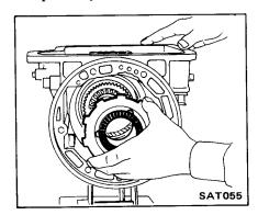
15. Install rear planetary carrier snap ring.
