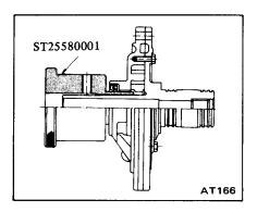
9. Set run-out of the cover to within specified total indicator reading.
