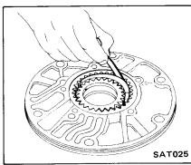
5. Measure clearance between outer gear and pump housing.
