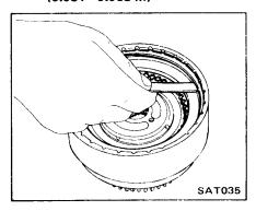
Test forward clutch (Rear)
