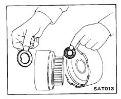
14. Remove forward clutch (Rear) hub, front planetary carrier and connecting shell, rear clutch thrust bearing, front planetary carrier thrust washer and thrust bearing.
