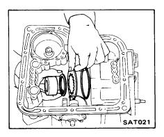
4. Align and start hex-head slotted bolts into inner race from rear of case.
