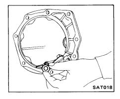
25. Remove one-way clutch inner race, return thrust washer, low and reverse return spring, and spring thrust ring.
