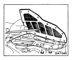
9. Check separator plate for scratches or damage. Replace if necessary. Scratches or score marks can cause oil to bypass correct oil passages and result in system malfunction.
