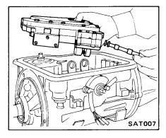
8. Loosen band servo piston stem locknut and tighten piston stem to prevent high-reverse clutch (Front) drum from dropping out when removing front pump.
