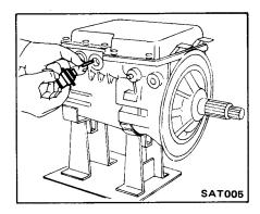
5. Remove speedometer lock plate retaining bolt. Remove speedometer pinion.
