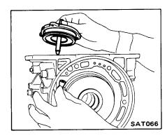
19. Install and torque the retainer bolts. Loosen piston stem.
