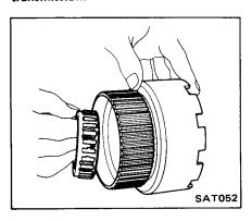
14. Secure thrust bearing and thrust washer with petroleum jelly and install rear planetary carrier.
