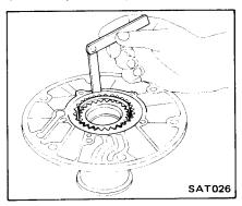
6. Using a feeler gauge and straight edge, measure clearance between gears and pump cover.
