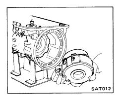
To prevent brake linings from cracking or peeling, do not stretch the flexible band unnecessarily. Before removing the brake band, always secure it with a clip as shown in the figure below.
