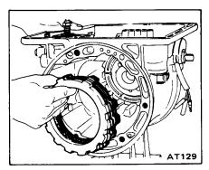
6. After low and reverse brake has been completely assembled, measure clearance between snapring and retainer plate. If measurement exceeds specifications it can be adjusted by replacing retainer plate with one of a different thickness.
